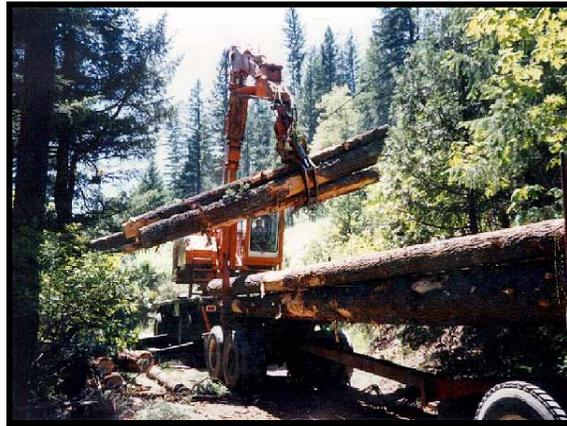
*A heeled boom loader is used to load logs on a narrow road, similar to roads found on the plan area. Specialized equipment such as this can be used to eliminate landings and reduce other impacts of logging.*
